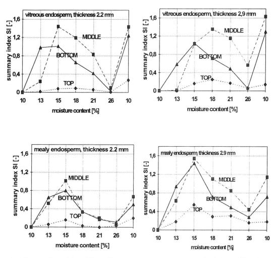
Fig. 1. Summary damage index as influenced by moisture content for the three zones of grain (top, middle and bottom), two endosperm structure (vitreous and mealy) and two grain size (thickness 2.2 and 2.9 mm).
